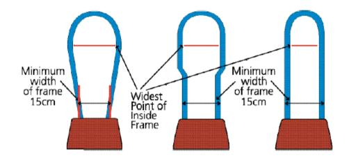
d) The frame may be fitted with a maximum of (4) four cross members, and one foot rail, mounted forward of the seat. The cross members may be square or cylindrical and not have a diameter smaller than 1.5cm or greater than 3cm.
