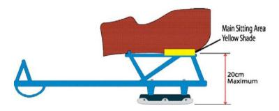
b) The maximum height a seat may sit above the ice is **20cm**, measured from a flat surface to the lowest point of the underside of the main seating area of the seat (See diagram below).
