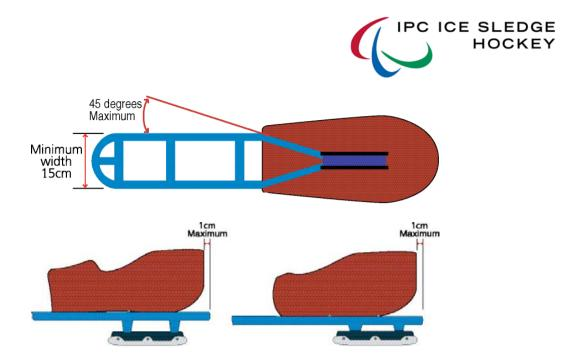
c) The front of the sledge shall have a continuous curve with a maximum radius **one half (1/2)** of the inside width of the frame at its widest point forward of the seat.
