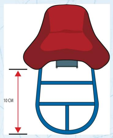
The area from the bottom of the side rails frame tubing to the ice must be a minimum of 8.5 cm and a maximum of 9.5 cm. The area behind the end of skag and in front of the blade and blade hold carrier must be free and clear. No padding or construction of any kind may cover this area.
