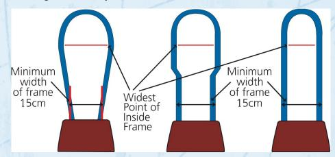
The frame may be fitted with a maximum of (4) four cross members, and one foot rail, mounted forward of the seat. The cross members may be square or cylindrical and not have a diameter smaller than 1.5cm or greater than 3 cm.
